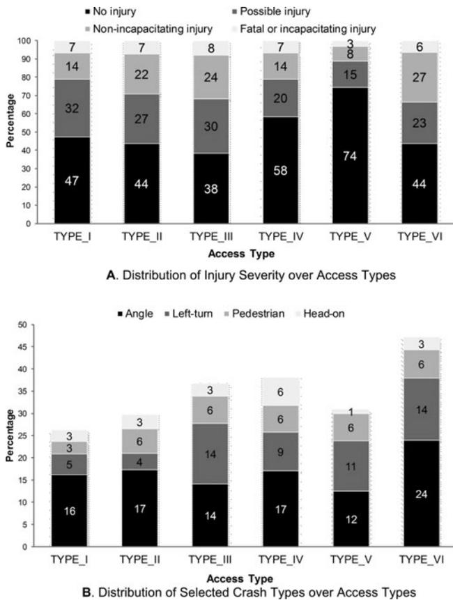
Fig. 3. Distributions of crash injury severity and selected crash types over 6 access types.
