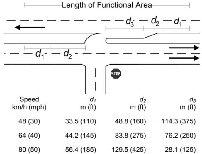
Fig. 2. Functional area of access points. Length of functional area is sum of perception reaction distance ( $d_1$ ), maneuver distance ( $d_2$ ), and storage length ( $d_3$ ) for both directions. Source: *Access Management Manual* (2003; table 8-4).
