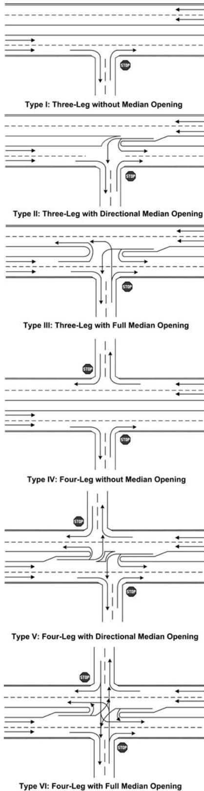
Fig. 1. Access designs and allowed movements at mid-block segments of multilane highways.
