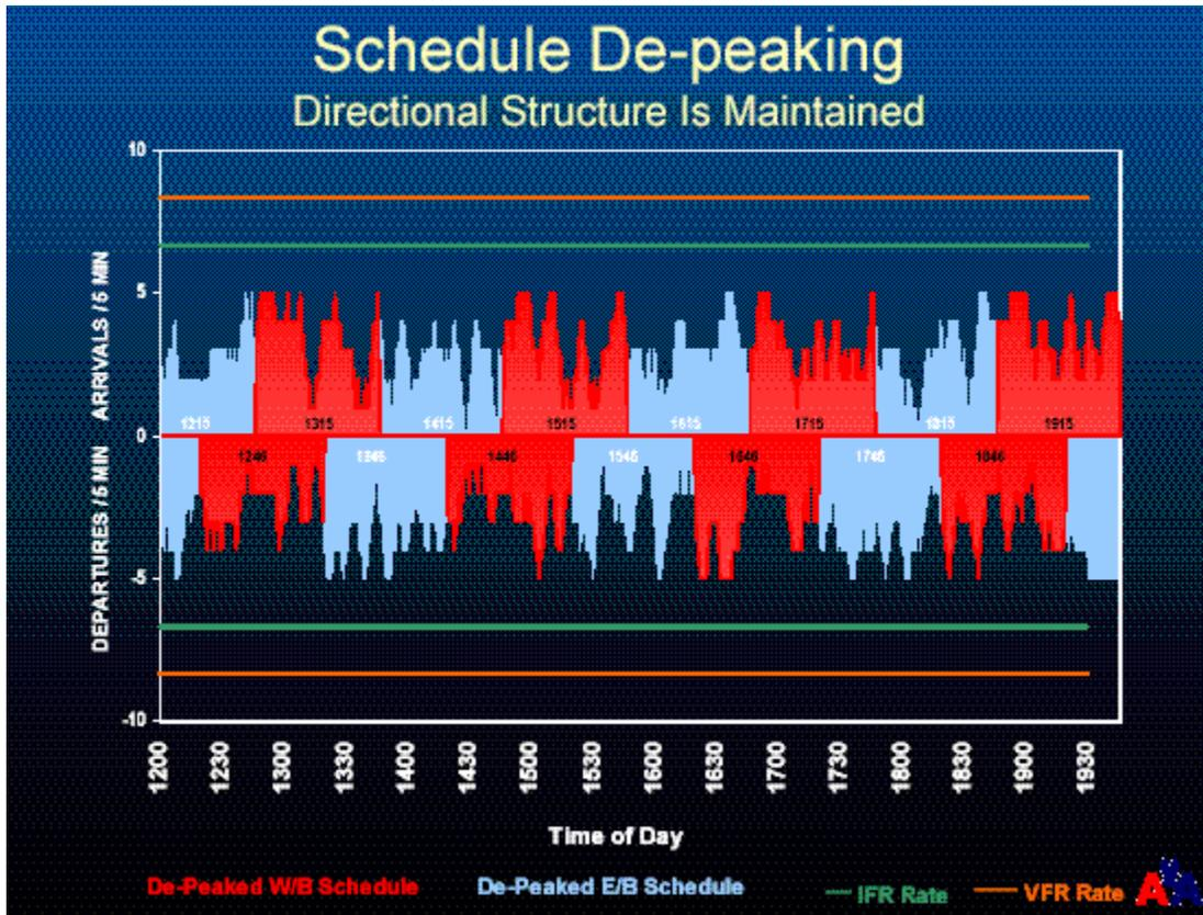
**FIGURE 2** Directional banks after depeaking.
